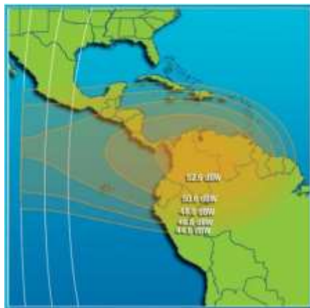
Fig 4 Huella de Cobertura IS 907.
