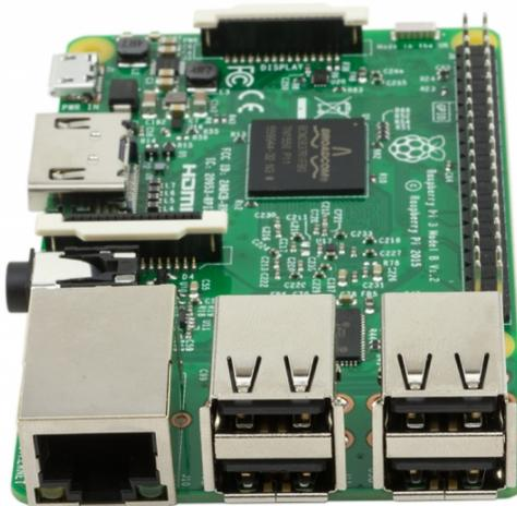
On top of all that, the low-level peripherals on the Pi make it great for hardware hacking. The 0.1" spaced 40-pin GPIO header on the Pi gives you access to 27 GPIO, UART, I<sup>2</sup>C, SPI as well as 3.3 and 5V sources. Each pin on the GPIO header is identical to its predecessor the Model B+.
