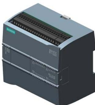
SIMATIC S7-1200, CPU 1214C, CPU COMPACTA, DC/DC/DC, E/S INTEGRADAS: 14 DI 24V DC; 10 DO 24 V DC; 2 AI 0 - 10V DC, ALIMENTACION: DC 20,4 - 28,8 V DC, MEMORIA DE PROGRAMA/DATOS 100KB
