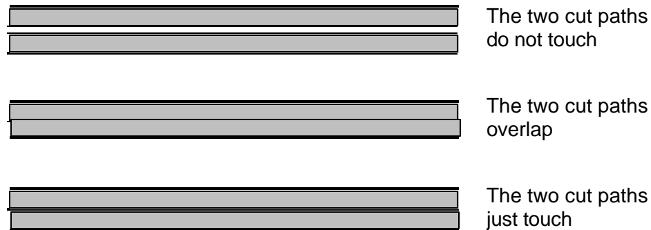
Figure 16 - Inspecting Mill Paths
